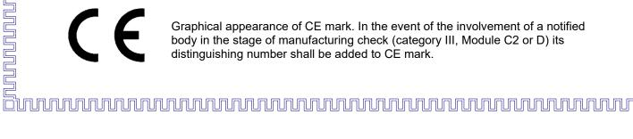
Graphical appearance of CE mark. In the event of the involvement of a notified body in the stage of manufacturing check (category III, Module C2 or D) its distinguishing number shall be added to CE mark.
